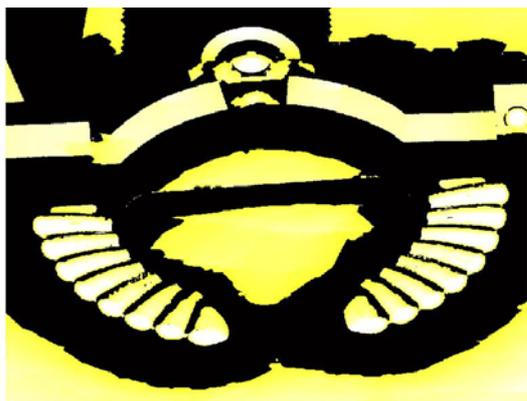
Figure 8 Annual irradiation falsecolour plot, thresholded to identify surfaces with good PV potential.
