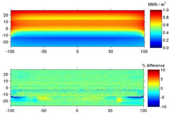
Figure 5 Annual irradiation for a diffuse sky with binned suns (upper) and associated difference plot (lower)
