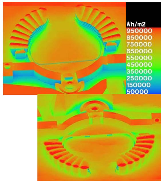
Figure 7 Annual irradiation falsecolour plot to identify surfaces with high solar exposure
