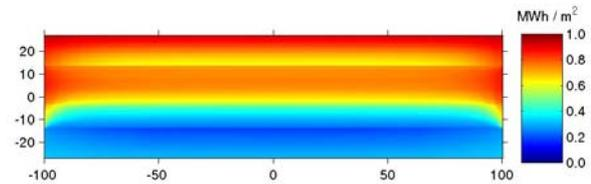
Figure 3 Annual irradiation throughout a 27m wide x 200m long canyon of  $h/w=1/2$ , located in Oslo (N.B. x, y axes relate to distance from centre of canyon).
